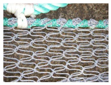
Section of a T90 extension showing consistent mesh opening
