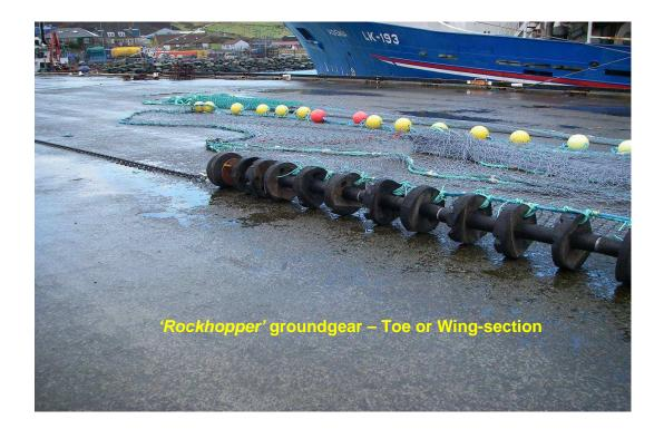
The *toe-end* of the groundgear was finished off with a *'bumper-bobbin'* arrangement forming the connection to the groundgear extension chains (2 x ~10.5m x 16mm mid-link) via a 12" *'bouncer pin'*. (See photos for details).
