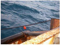
SCANMAR distance sensor on trawl door
