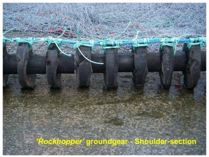
The wing sections (x 2) consisted of 16 x 16" (406mm) discs with 2 x 7"x 5" (178mm x 127mm) spacers between each disc except for the last two discs in each section which were separated by one spacer. Additional weight was added as for the other two sections.
