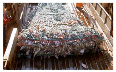
T90 codends with catch onboard Icelandic vessel
