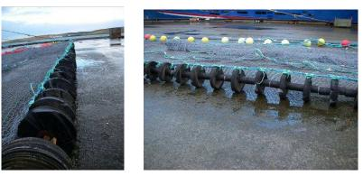
The mid-section consisted of  $1 \times 19'10''$  (~6.0m) length of 24mm wire with 24 x 18'' (457mm) rubber *'Rockhopper'* discs. The discs were separated by 1 x 7'' x 7'' (178mm x 178mm) rubber spacers. Extra weight in the form of 6 x 2kg lead washers was evenly distributed over the length of the centre section.
