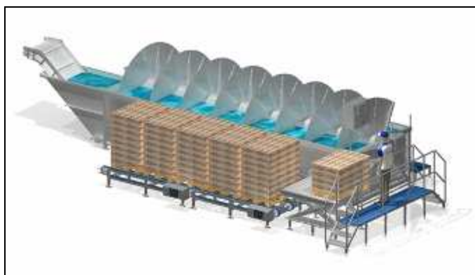
Figure 18 - Example of modern design of water based thawing unit (GW Containers)
