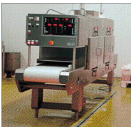
Figure 16 - Example of a continuous RF tunnel (50kW, 750 to 2000kg/hour) (Sairem S.A.)
