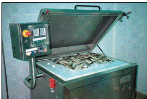
Figure 15 - Example of a batch RF thawing/tempering system (6kW, 100 to 250 kg/hour) (Sairem S.A.)
