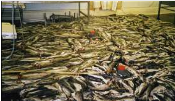
a) Frozen fish blocks set out on the floor and using a 'garden sprinkler' water spray
