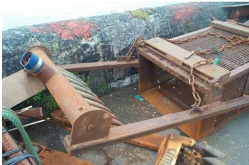
Figure 2.3 Ensis dredge operated on Balbriggan vessel
