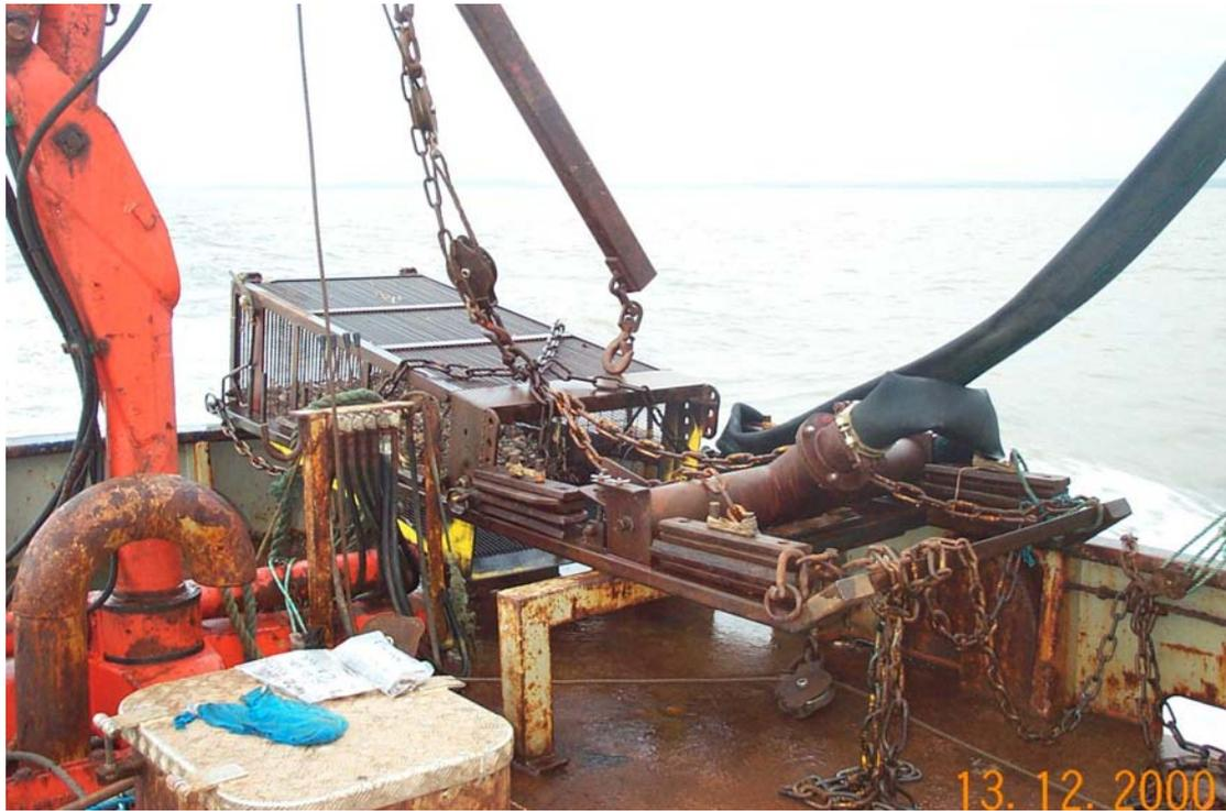
Figure 3.1. a The experimental dredge constructed for use in the field trials in The Wash
