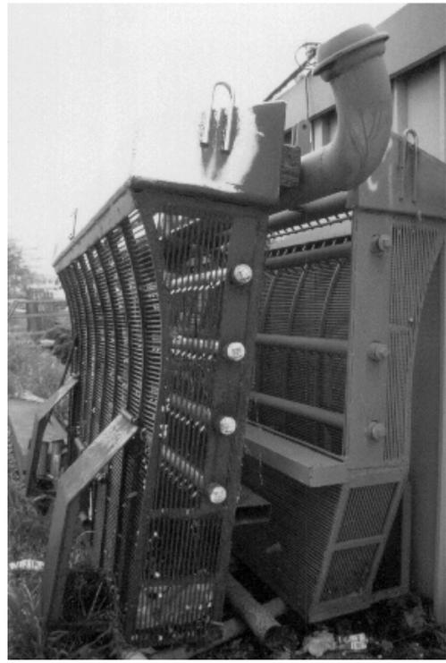
Figure 3.17 Hydraulic dredge for *Ensis siliqua minor* by M. Pellizzato
