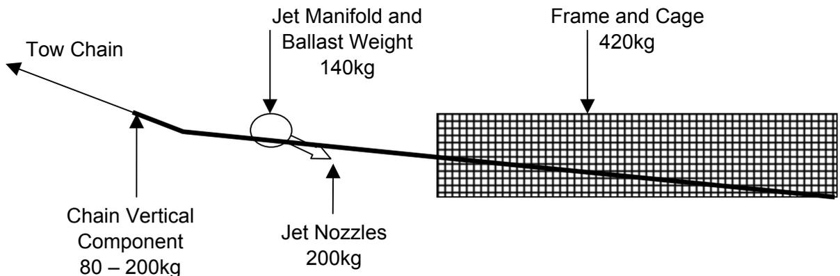
**Figure 8 : Weight and Vertical Forces Acting on the Dredge**
