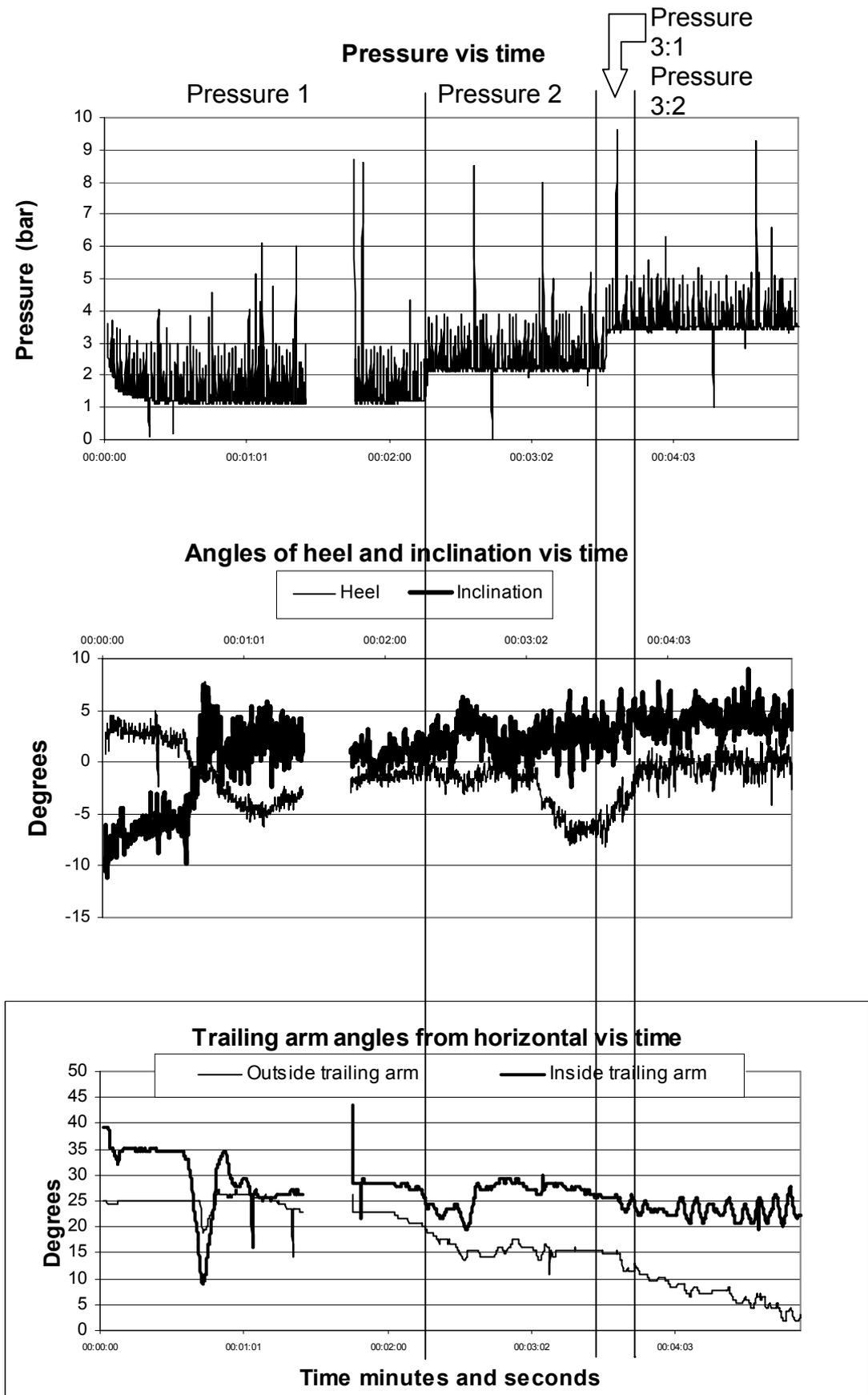
Figure 3.9 Instrumentation Data from haul on Seal Sand site. Vertical lines correspond to stages in Table 3.4 and Figures 3.11-3.14
