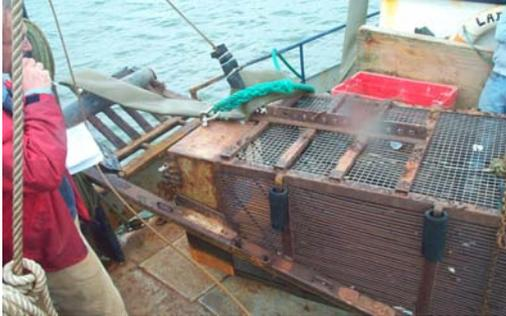
Figure 2.2 Ensis dredge operated on Skerries vessel
