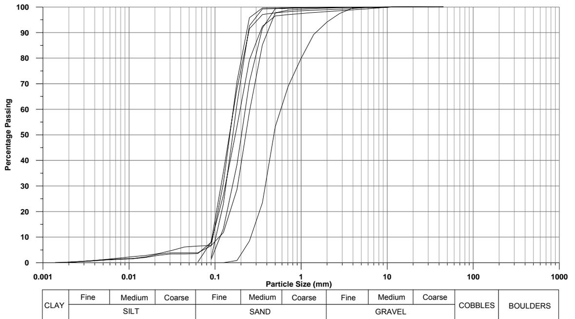
**Figure 4: Grab-sampled Particle Size Distribution Results**
