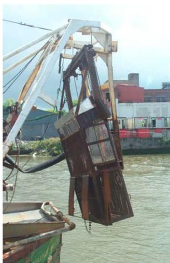
Figure 2.1 Ensis dredge operated on Drogheda vessel
