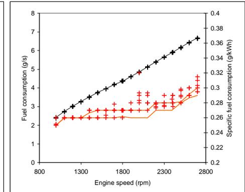
Full Figure 19: Baseline archive plot of tests Baseline\_002\_014 to Baseline\_002\_019 inclusive, showing engine performance envelope defined by Baseline\_002\_008 to Baseline\_002\_013. Solid, black line – Baseline 002\_015 performance. With progressive testing, problem became worse. p84 in main report
