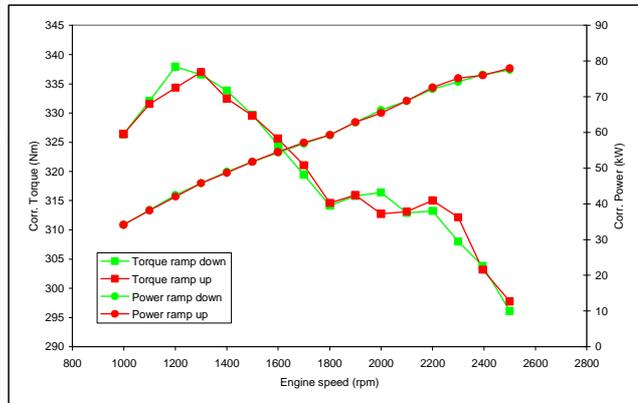
CSM Marine Diesel Engine Test Cell
