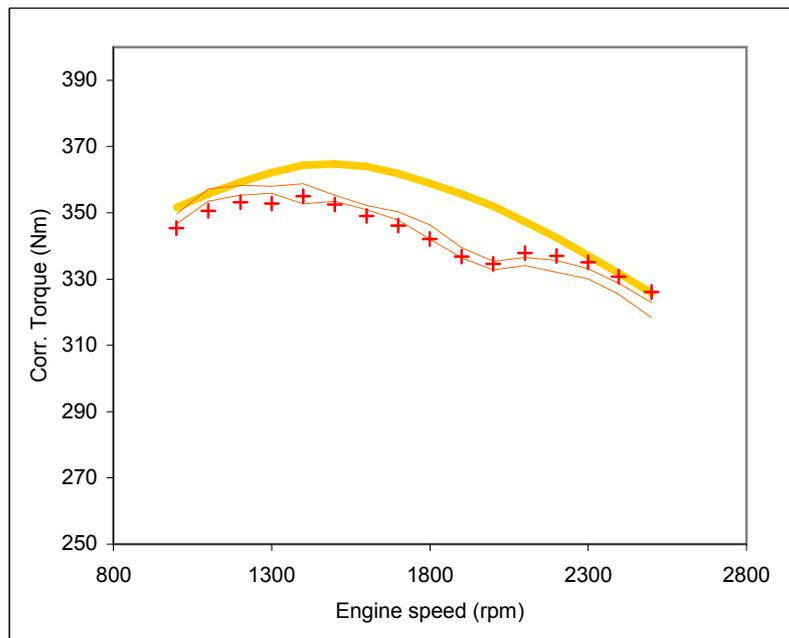
**Figure 24: Post additive A Baseline test performance with engine performance envelope defined by Baseline 003\_108, Baseline 003\_109, Baseline 003\_114 and Baseline 003\_118.**
