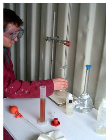
**Figure 6: Titration in progress**
