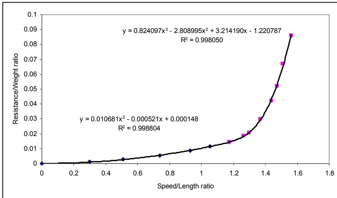
**Figure 11: Resistance curve for a generic displacement hull (based on formulation presented by Savitsky, 2003).**
