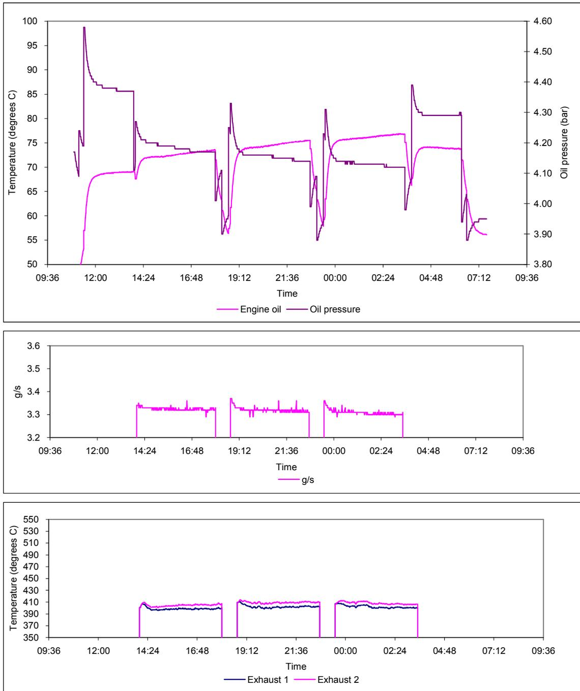
**Figure 35: Oil temperature, oil pressure, fuel consumption and exhaust gas temperature for test 107 fuelled using fossil diesel with no additives.**
