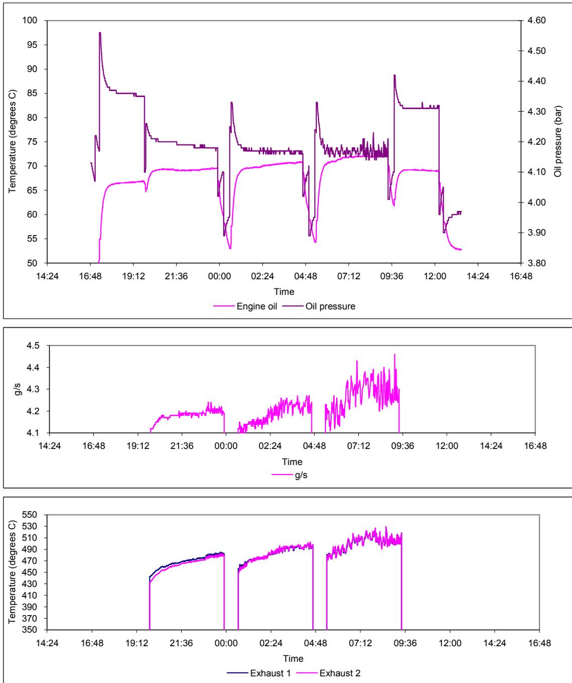
**Figure 38: Oil temperature, oil pressure, fuel consumption and exhaust gas temperature for test 113 fuelled using waste oil (RVO) derived biodiesel. This was the last test conducted prior to it being discovered that the engine had suffered a failure.**
