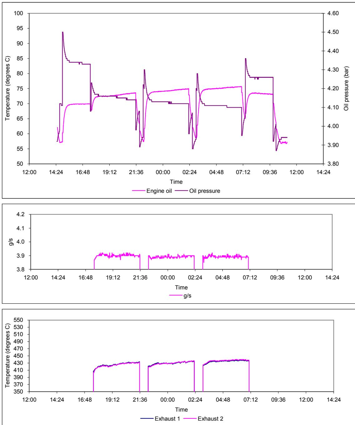
**Figure 37: Oil temperature, oil pressure, fuel consumption and exhaust gas temperature for test 112 fuelled using BS14214 methyl ester.**
