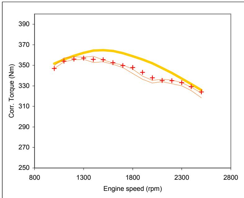
**Figure 26: Post additive C Baseline test performance with engine performance envelope defined by Baseline 003\_108, Baseline 003\_109, Baseline 003\_114 and Baseline 003\_118.**
