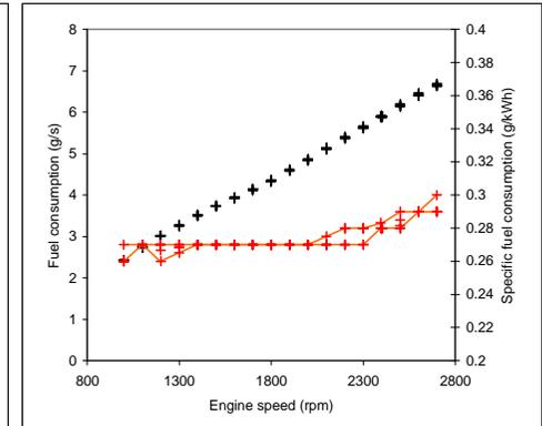
Full Figure 17: Baseline archive plot of tests Baseline\_002\_001 to Baseline\_002\_007 inclusive, showing engine performance envelope defined by these tests. p82 in main report
