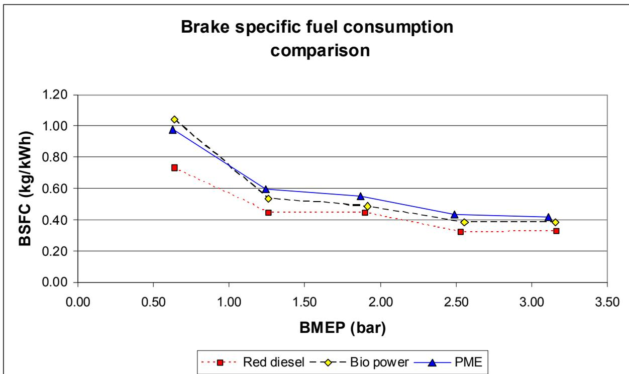
**Figure 08: Preliminary fuel consumption tests from the test cell, with petrodiesel, palm methyl ester and ‘Biopower V100’ (sunflower oil with a propriety additive).**
