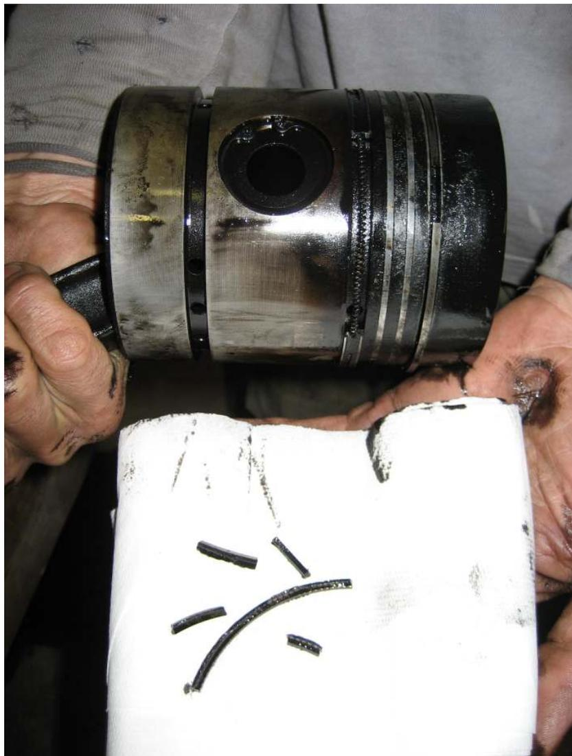
**Figure 02: Broken and seized piston rings**
