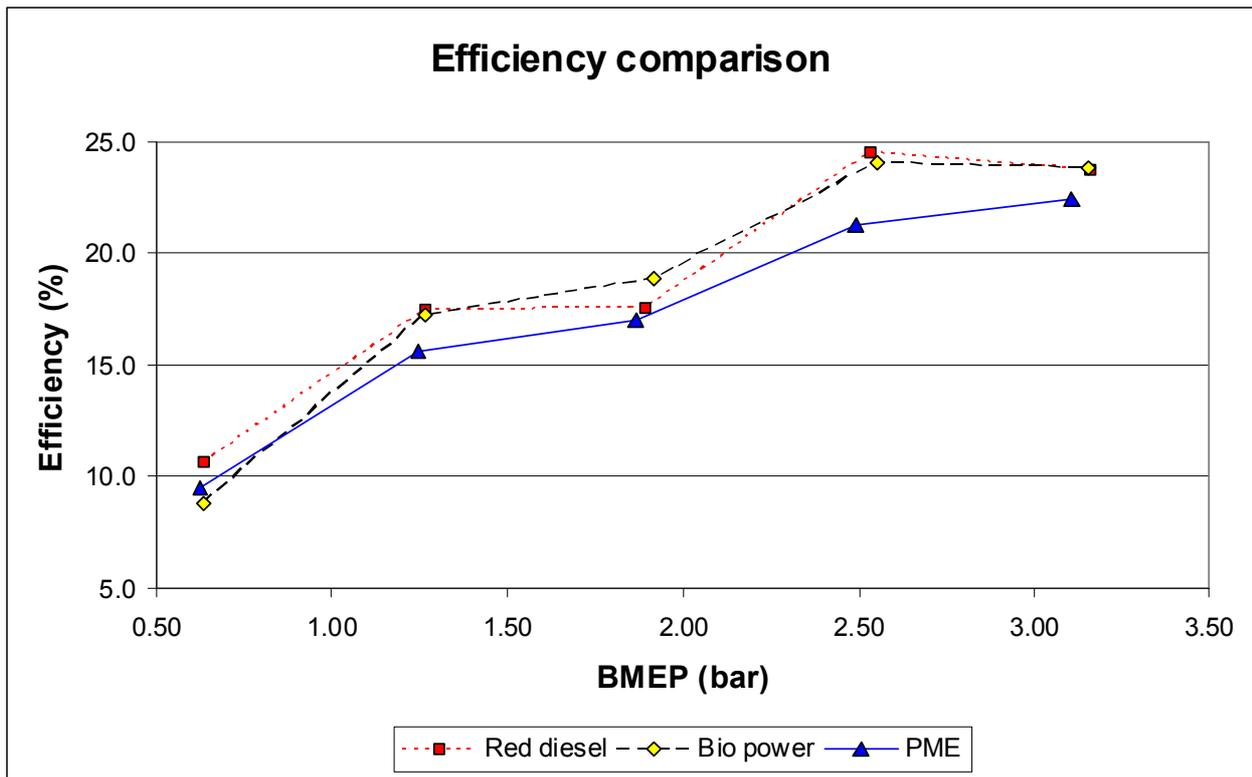
**Figure 09: Preliminary efficiency tests from the test cell, with petrodiesel, palm methyl ester and ‘Biopower V100’ (sunflower oil with a propriety additive).**
