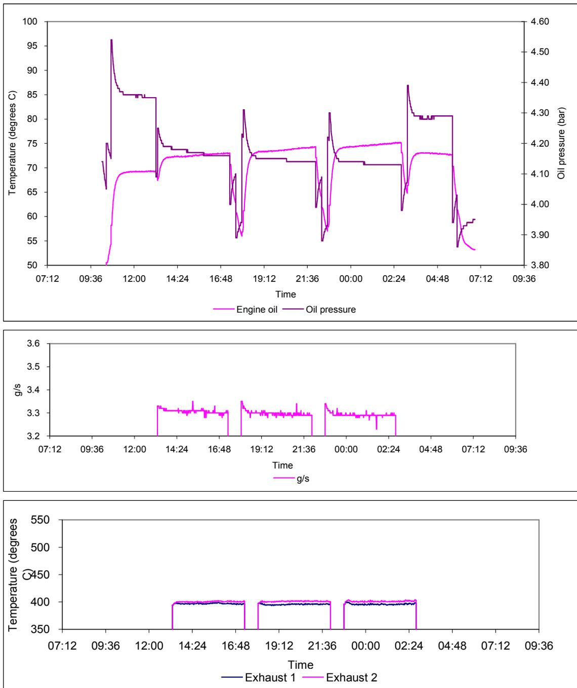
**Figure 36: Oil temperature, oil pressure, fuel consumption and exhaust gas temperature for test 111 fuelled using fossil diesel with no additives. This was the last DayTrawl test conducted prior to testing biofuels.**
