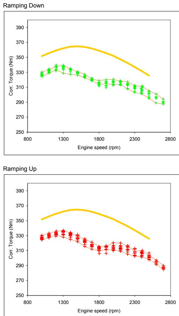
**Figure 20: Baseline archive plot of Baseline 003\_001 to Baseline 003\_006 showing engine performance envelope defined by Baseline\_002\_008 to Baseline\_002\_013**
