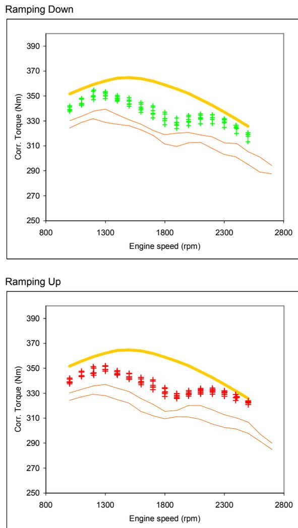
**Figure 22: Showing engine performance envelope defined by Baseline\_002\_008 to Baseline\_002\_013 and Baseline 003\_001 to Baseline 003\_006 with Baseline 003\_101 to Baseline 003\_107 performance data shown as discrete points.**
