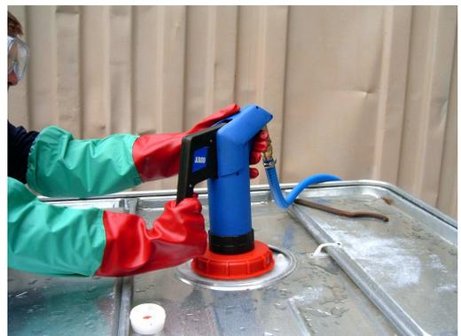
**Figure 8: Fitting the methanol pump**
