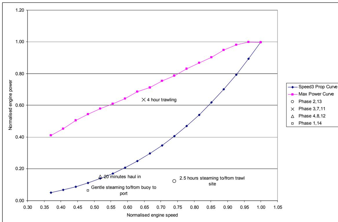
**Figure 12: Normalised maximum power curve for 6 cylinder Perkins 6.3544M engine in CSM Test Cell together with phase set points for proposed day boat trawler cycle and cubic propeller law relating engine speed to power (as in EPA, 1998).**
