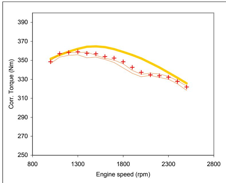
**Figure 25: Post additive B Baseline test performance with engine performance envelope defined by Baseline 003\_108, Baseline 003\_109, Baseline 003\_114 and Baseline 003\_118.**
