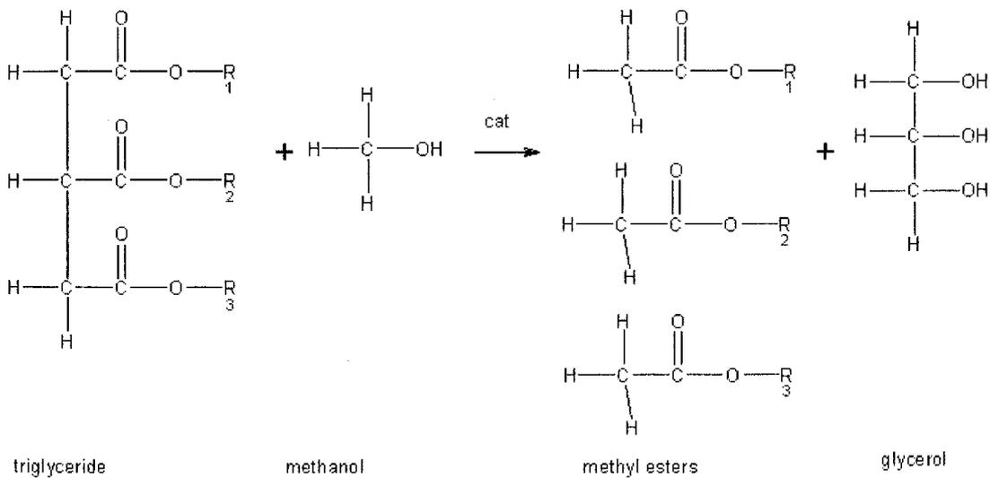
**Figure 05: The transesterification of vegetable oil using methanol.**
