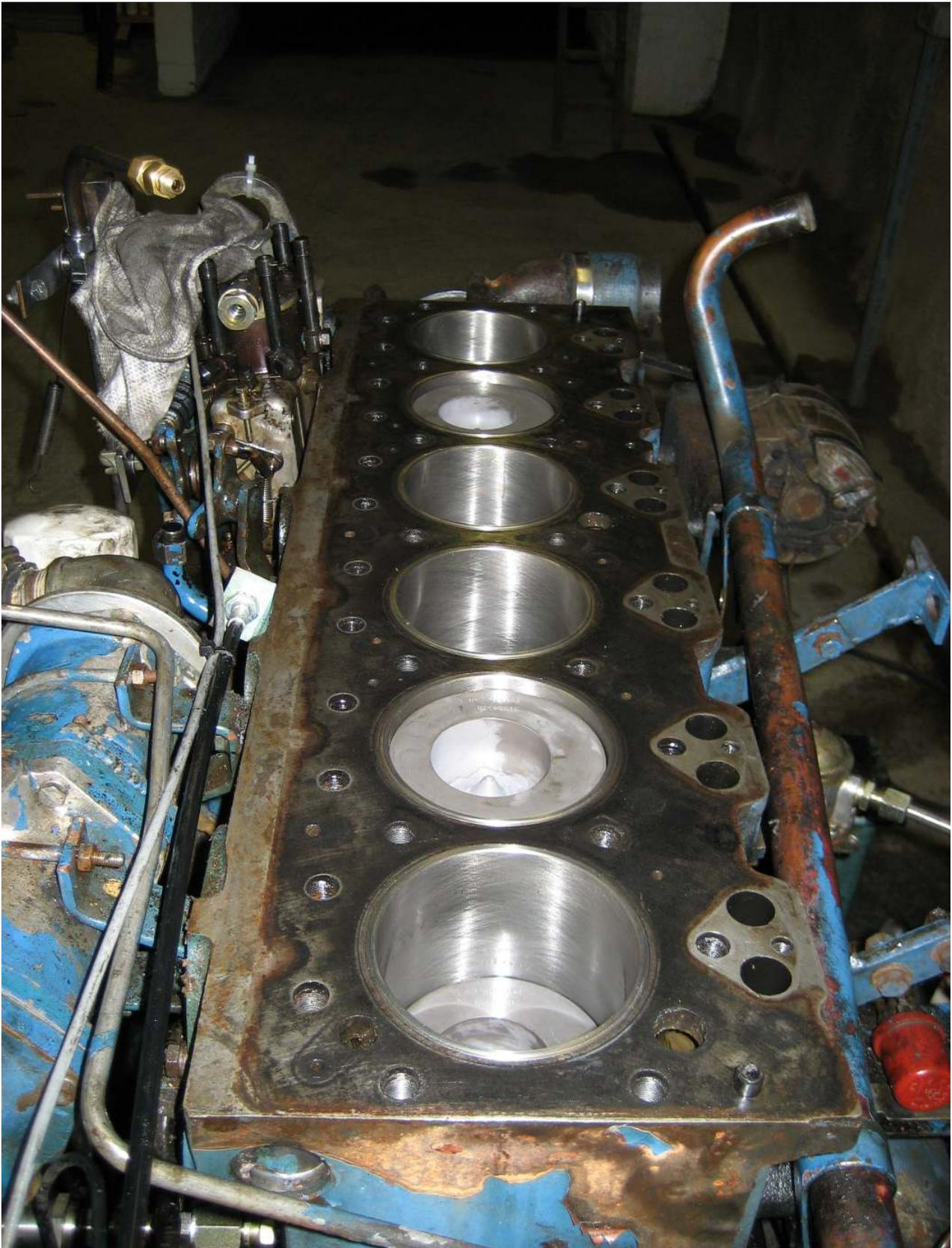
**Figure 03: New cylinder liners and pistons**
