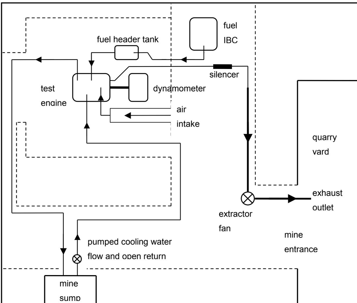
Figure 01: Schematic diagram of test infrastructure within the mine.
