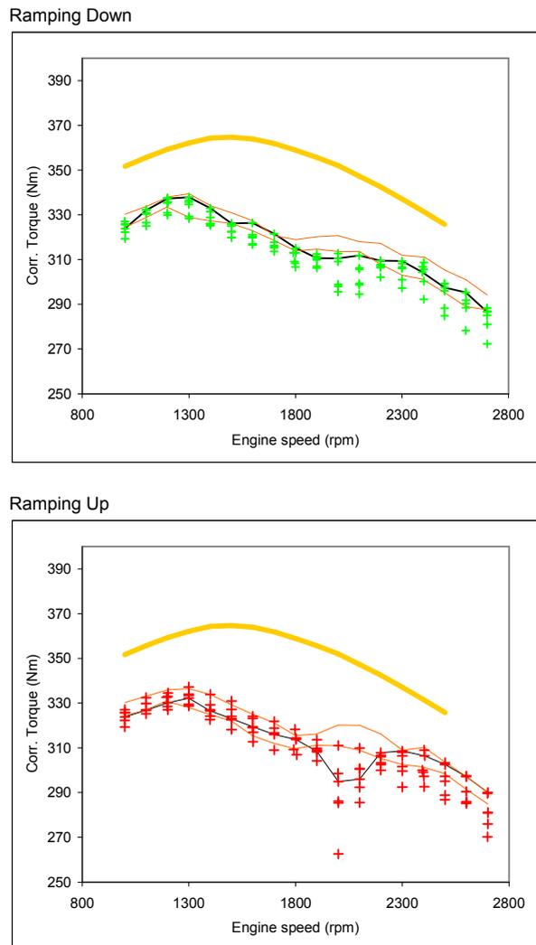
**Figure 19: Baseline archive plot of tests Baseline\_002\_014 to Baseline\_002\_019 inclusive, showing engine performance envelope defined by Baseline\_002\_008 to Baseline\_002\_013. Solid, black line – Baseline 002\_015 performance. With progressive testing, problem became worse.**
