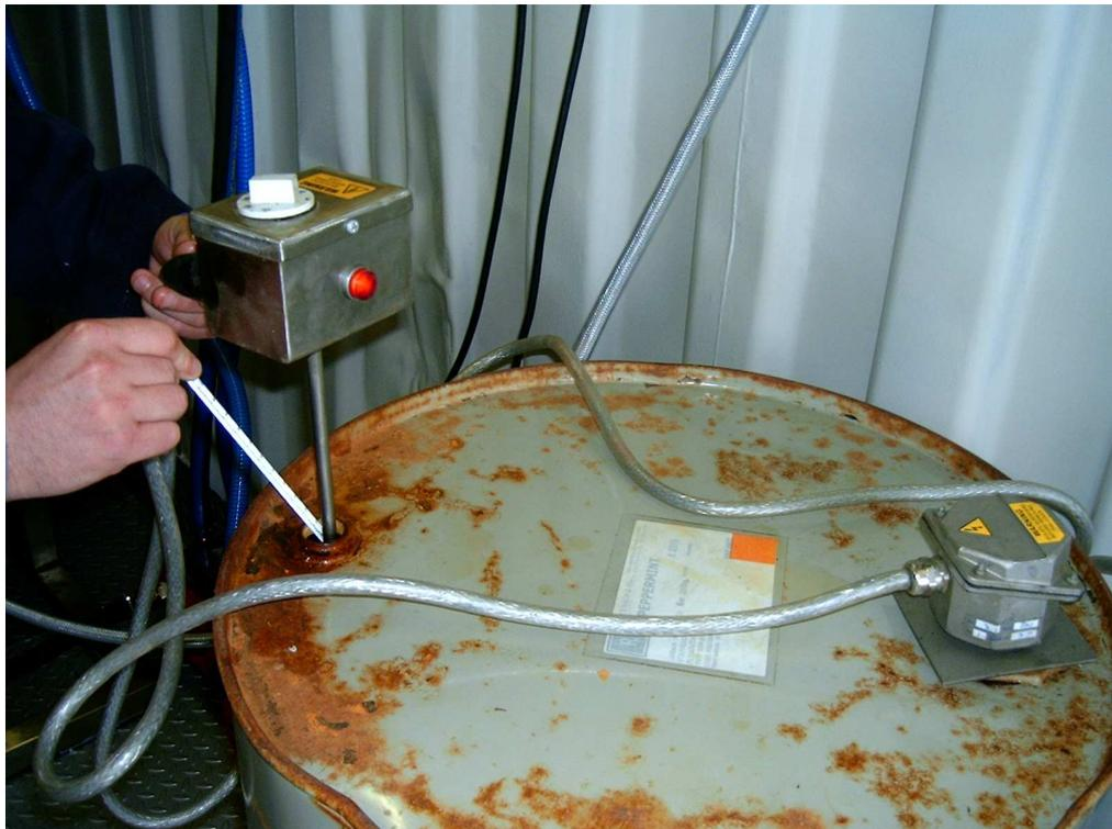
**Figure 7: Lifting the thermostat slightly to measure the temperature at the top of the barrel. Note that the red light is lit showing that the thermostat is calling for heat.**
