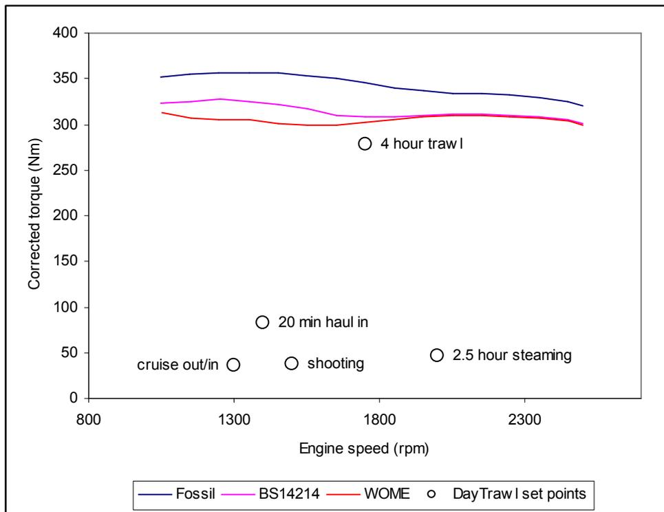
**Figure 39: Torque curves (average of ramp down and ramp up) for fossil diesel, BS14214 biodiesel, and waste oil methyl ester (WOME), also showing DayTrawl stage set points.**
