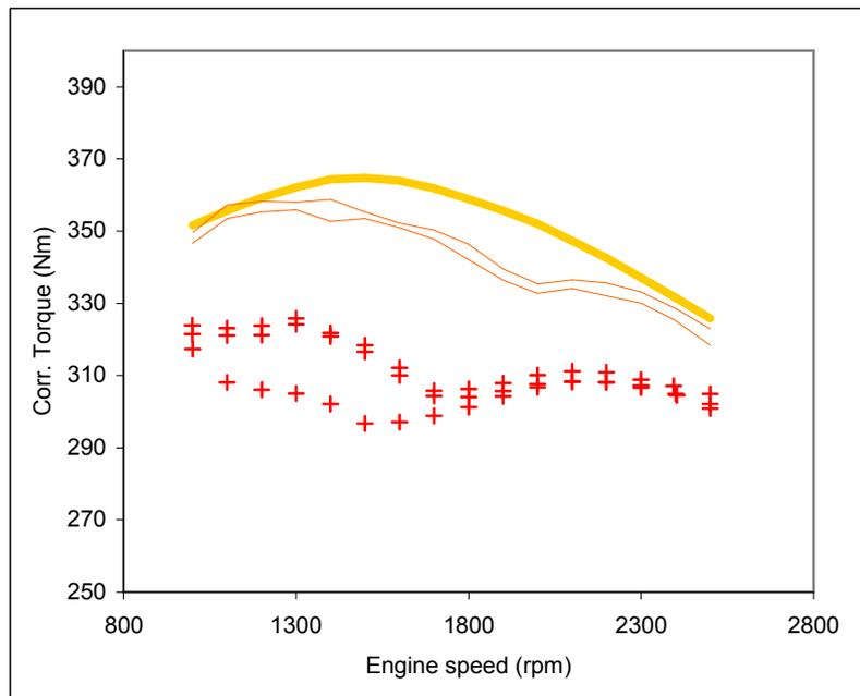
**Figure 32 : Baseline 003\_119\_ME, Baseline 003\_120\_ME and Baseline 003\_121\_WO test performance with engine performance envelope defined by Baseline 003\_108, Baseline 003\_109, Baseline 003\_114 and Baseline 003\_118.**
