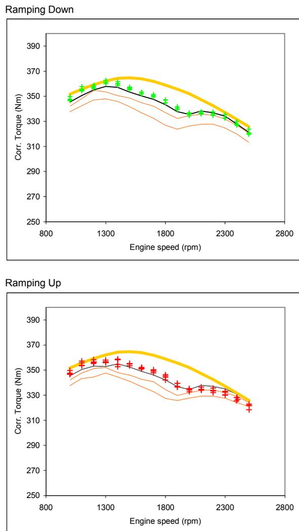
**Figure 23: Baseline 003\_107 (solid line) together with the engine performance envelope established from Baseline 003\_101 to Baseline 003\_107 and results from Baseline 003\_108, Baseline 003\_109, Baseline 003\_114 and Baseline 003\_118 (clusters)**
