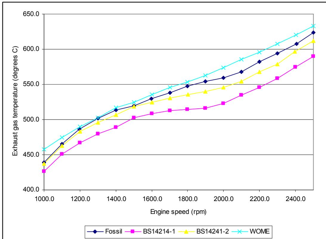
**Figure 34: Exhaust gas temperature from the ramping up sections of Baseline tests 118 (Fossil diesel) 119 (BS14214 methyl ester), 120 (BS14214 methyl ester) and 121 (waste oil methyl ester).**
