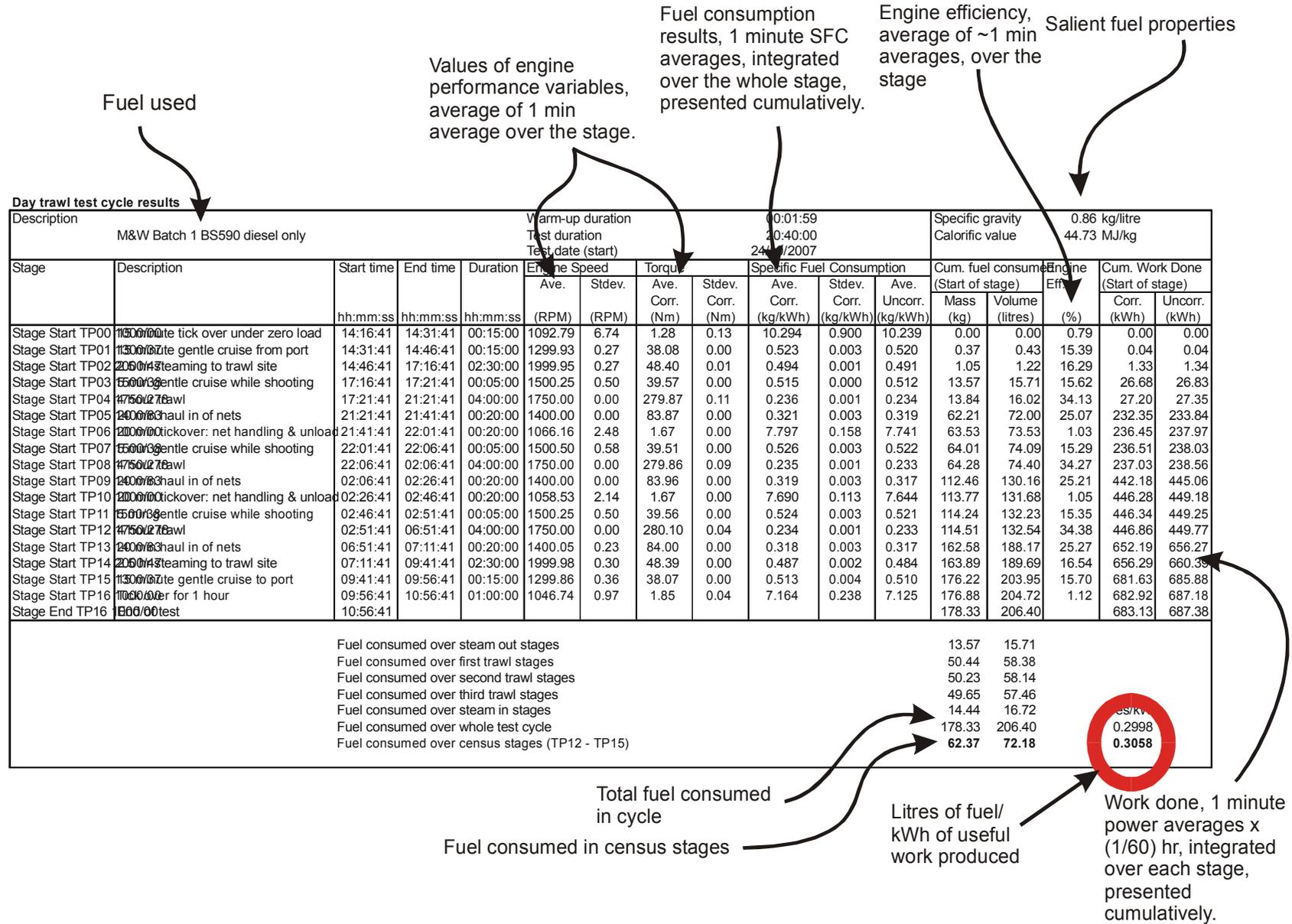
Figure 14 : Guide to tabular results format for DayTrawl test results
