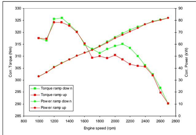
CSM Marine Diesel Engine Test Cell
