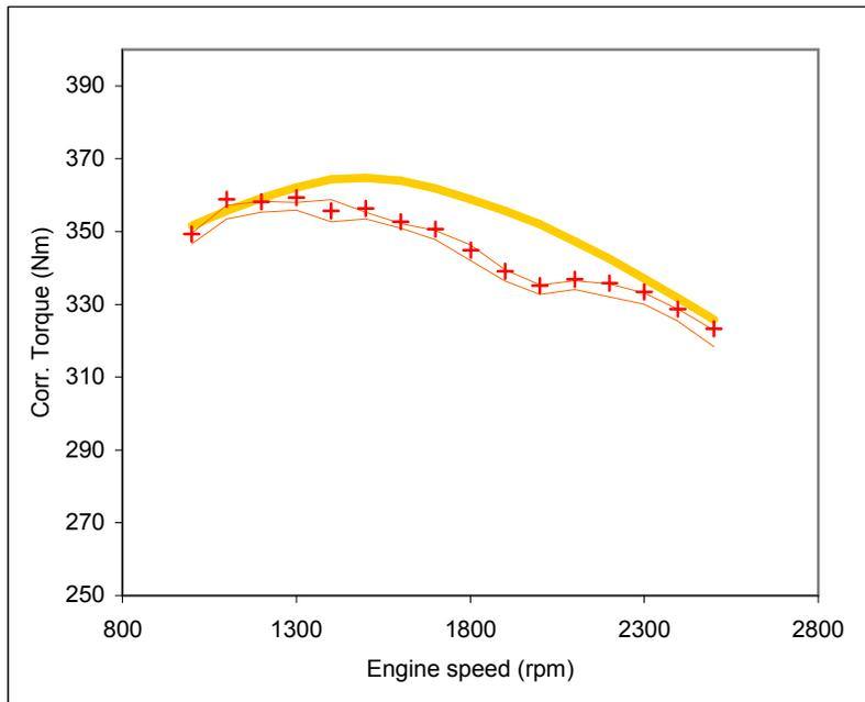
**Figure 28: Post additive E Baseline test performance with engine performance envelope defined by Baseline 003\_108, Baseline 003\_109, Baseline 003\_114 and Baseline 003\_118.**
