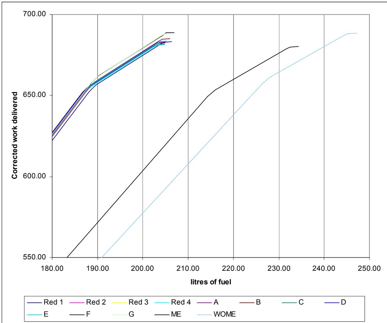
**Figure 33: Comparison between fuel / fuel + additive performance over the DayTrawl test cycle.**
