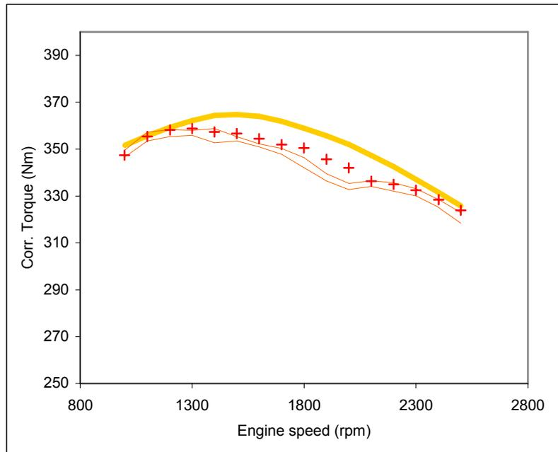
**Figure 27: Post additive D Baseline test performance with engine performance envelope defined by Baseline 003\_108, Baseline 003\_109, Baseline 003\_114 and Baseline 003\_118.**
