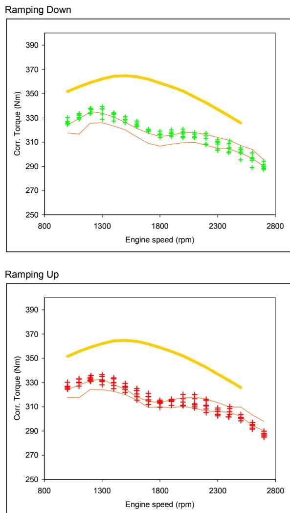
**Figure 18: Baseline archive plot of tests Baseline\_002\_008 to Baseline\_002\_013 inclusive, showing engine performance envelope defined by Baseline\_002\_001 to Baseline\_002\_007.**
