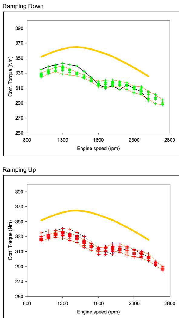
**Figure 21: Showing engine performance envelope defined by Baseline\_002\_008 to Baseline\_002\_013 and Baseline 003\_001 to Baseline 003\_006 with Baseline 003\_007 performance curve superimposed (solid black line).**
