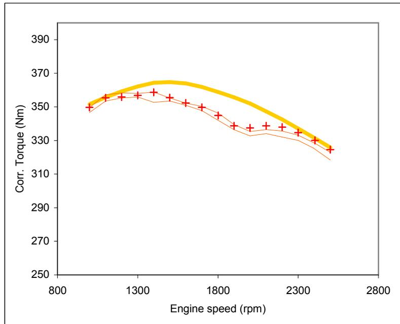
**Figure 30: Post additive G Baseline test performance with engine performance envelope defined by Baseline 003\_108, Baseline 003\_109, Baseline 003\_114 and Baseline 003\_118.**
