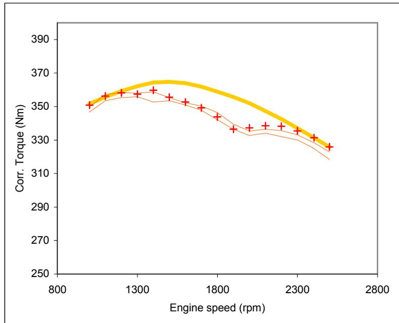
**Figure 29: Post additive F Baseline test performance with engine performance envelope defined by Baseline 003\_108, Baseline 003\_109, Baseline 003\_114 and Baseline 003\_118.**
