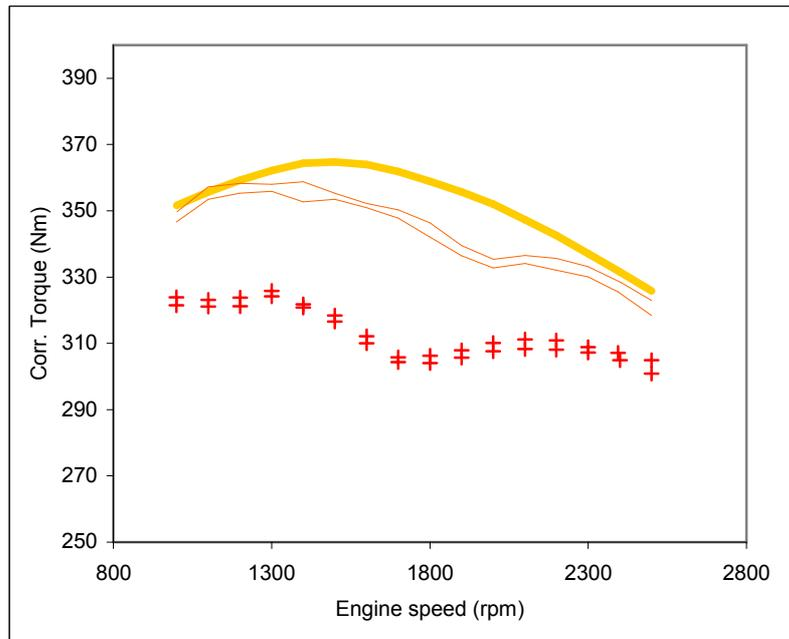
Figure 31 : Baseline 003\_119\_ME and Baseline 003\_120\_ME test performance with engine performance envelope defined by Baseline 003\_108, Baseline 003\_109, Baseline 003\_114 and Baseline 003\_118.
