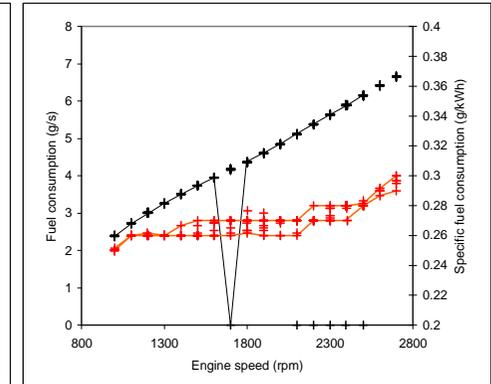
Full Figure 21: Showing engine performance envelope defined by Baseline\_002\_008 to Baseline\_002\_013 and Baseline 003\_001 to Baseline 003\_006 with Baseline 003\_007 performance curve superimposed (solid black line). p86 in main report
