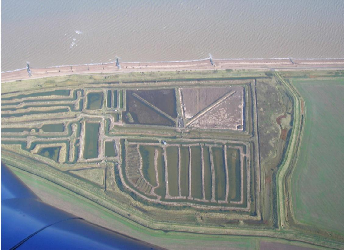
Once completed, any of these ponds will be capable of being emptied independently of the rest of the system and dried out. Thereafter, on refilling a good phytoplankton bloom will develop naturally and this can then be used to supply the rest of the nursery system.
