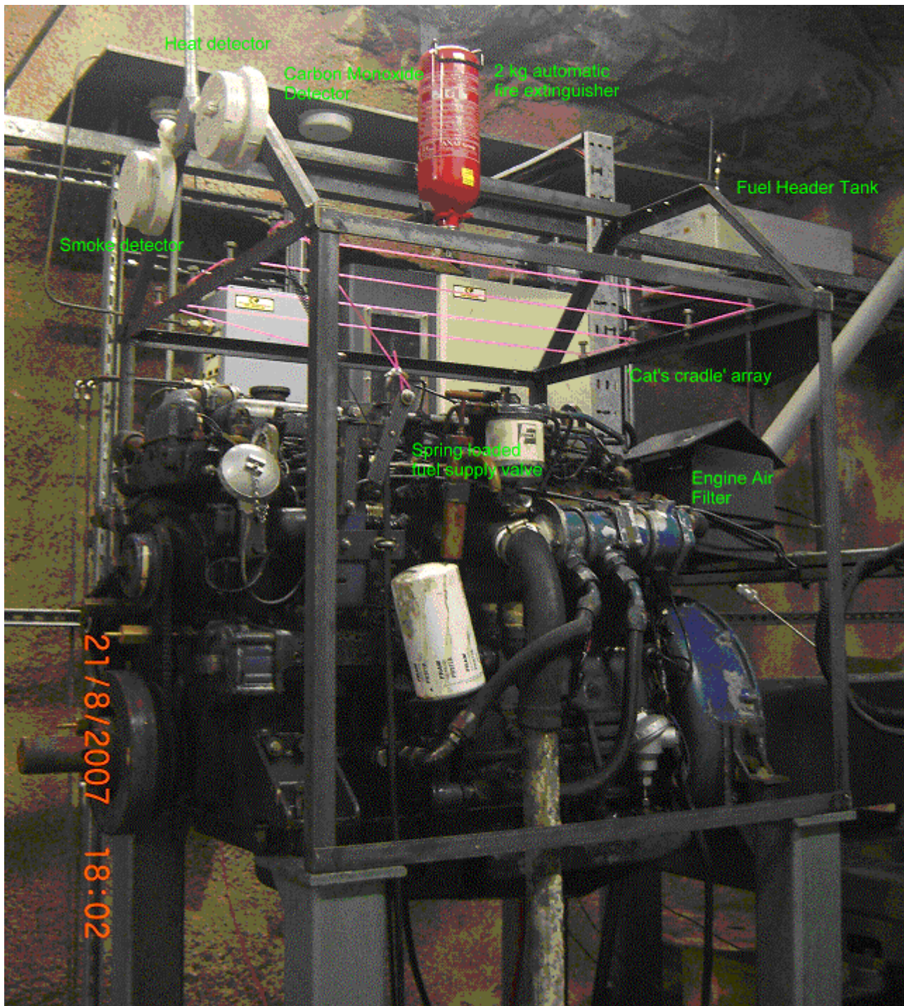
Figure 06: Test engine showing fire protection measures installed to support unattended operations for prolonged testing.
