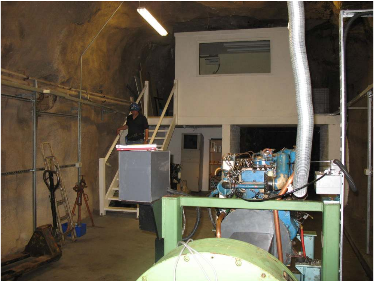
Figure 01: Photograph of the bio-fuel engine test cell facility underground at the CSM Holman's Test Mine. The top of the photograph shows the test cell control cabin. The dynamometer is in the foreground in green, the test cell engine is in blue.
