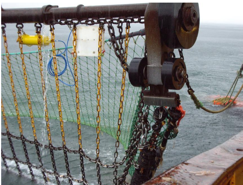
Camera and hard drive fitted to the down chains
