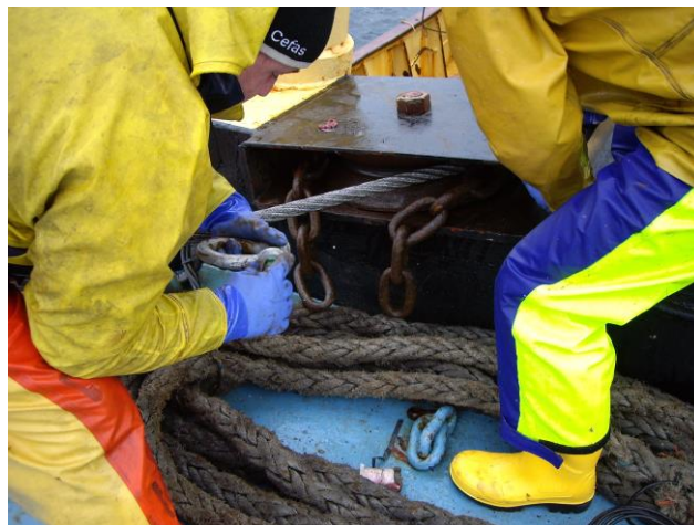
Load cells being fitted to the warps
