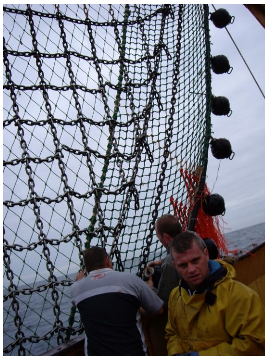
Replacing the rubbered wire footrope
