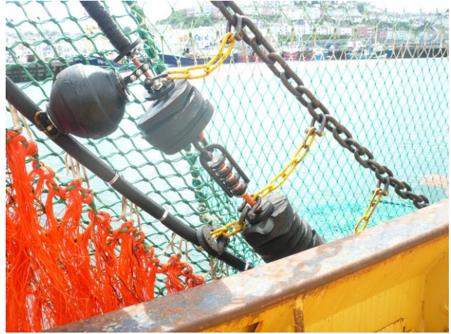
Rollerball & standard hopper ground gear
