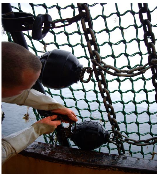
Rubber spans being fitted between the balls
