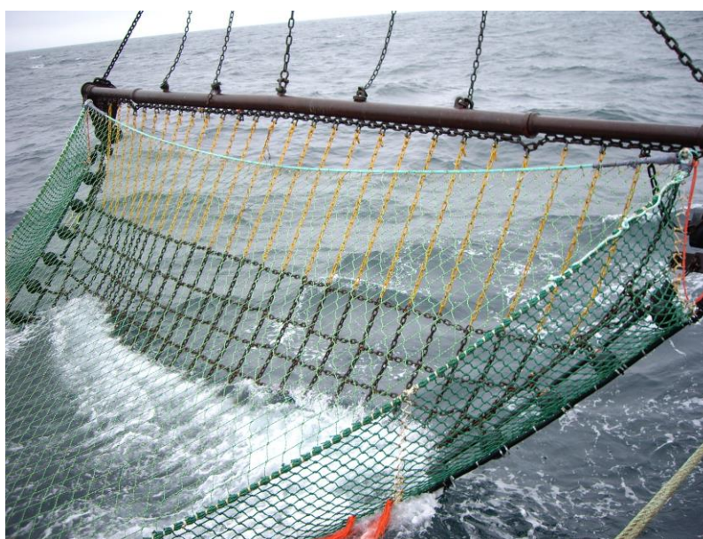
Rollerball gear in its current form
