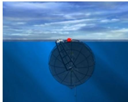
**Figure 40 Position 2:** Surface position or iceberg position, is the normal breeding position for all anadromous species. Approximately 10% of the system is above surface, so that the fish can get air from an air dome in top of the cage.
