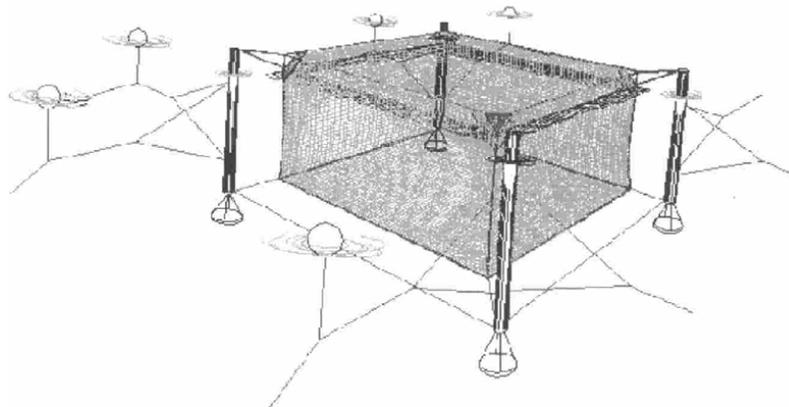
**Figure 31** Diagram of Ocean Spar net pen – note the spar bouys at each corner, against which the net is tensioned.
