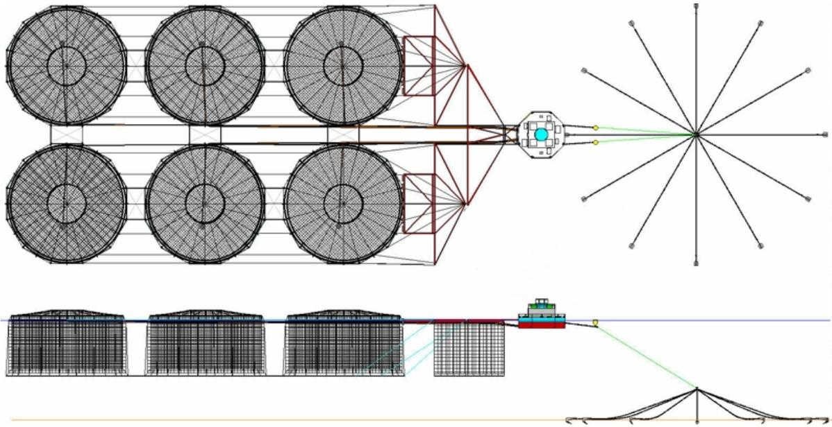
**Figure 25** Canadian Aquaculture Engineering Group (AEG – Canada). Above – plan view of six cages attached to framework and through a feed and service barge to a single point mooring system. Below – side view of system (<http://www.aquacultureengineeringgroup.com>).
