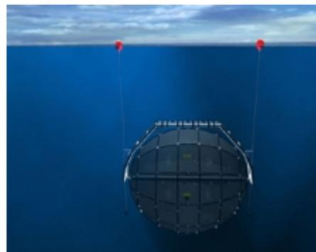
**Figure 42 Position 4:** Extreme-submerged, this position occurs in extreme situations like algae invasions, unfavourable temperatures, storms/typhoons etc. or if the bred fish naturally belongs in the deep water
