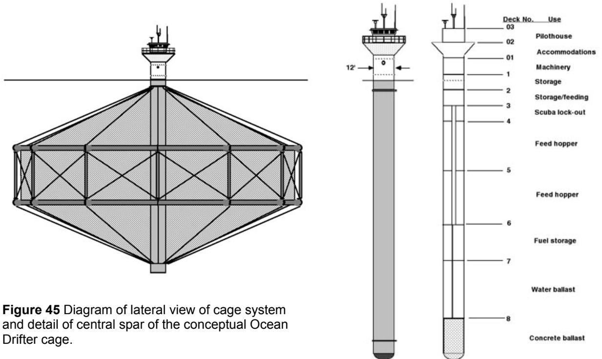
**Figure 45** Diagram of lateral view of cage system and detail of central spar of the conceptual Ocean Drifter cage.
