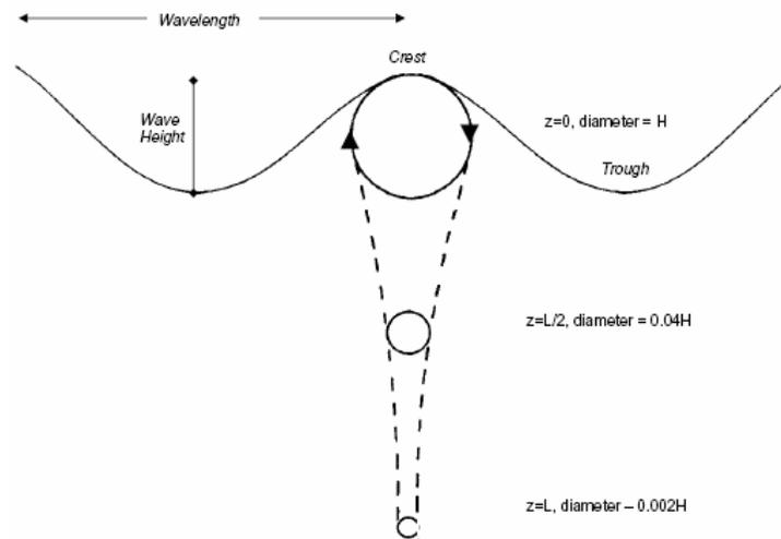
**Figure 21** Rotational properties of water particles in a wave (Modified after Pond and Pickard 1983)
