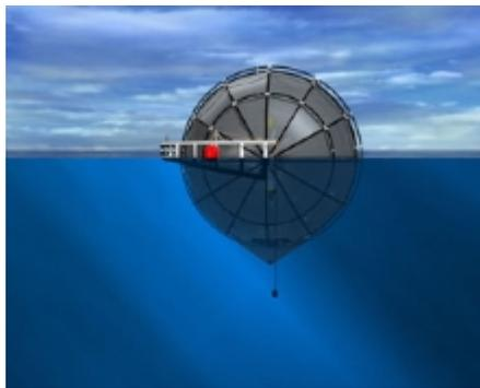
**Figure 39 Position 1:** Semi-Submerged is a working position. Personnel can safely do all the necessary work operations above the water from a horseshoe shaped working platform. Hence, no divers are needed
