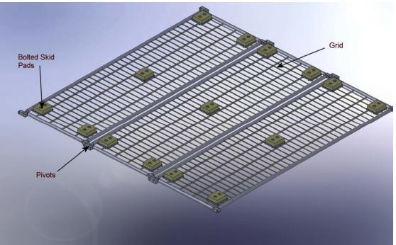
Figure 11: Wear pads bolted to proposed grid
