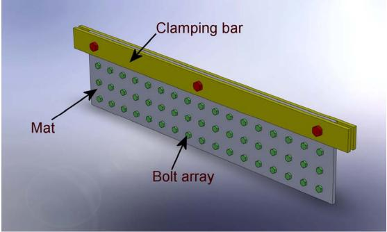
Figure 5: Wear pad arrangement
