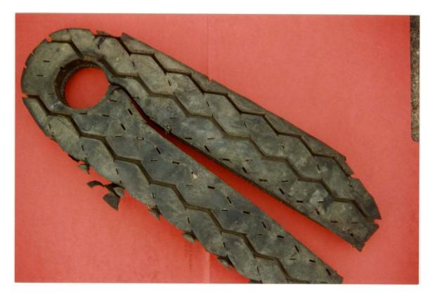
Scallop bucket made with 76 mm (3 inch) rings and steel washers and rubber pads (steel-pad).
