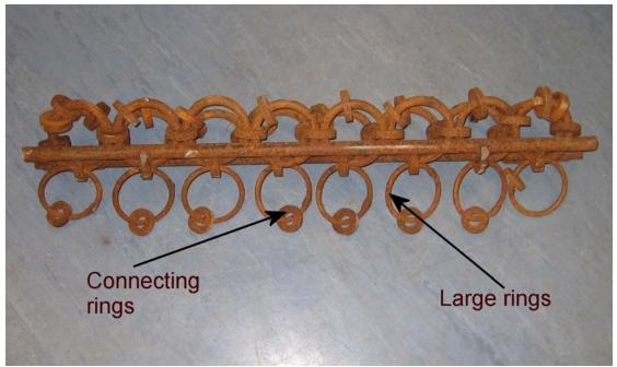
Figure 9: Section of current chain
