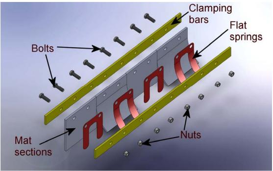
Figure 7: Flat spring stiffener arrangement
