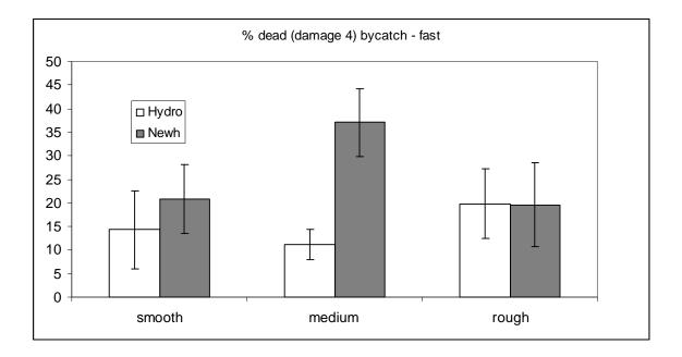
Figure 3. Percentage of bycatch showing damage score 4 (dead) in each of Hydro- and Newhaven dredges for three ground types (smooth, medium and hard) at each of slow (2.5kn) and fast (4.0kn) towing speeds.
