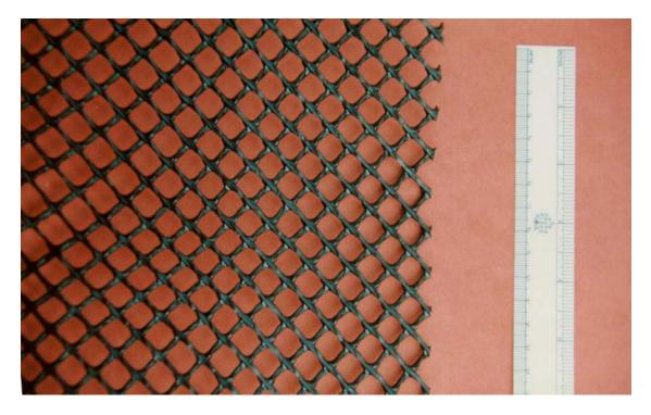
Vexar used to line two buckets made with 76 mm (3 inch) rings and steel washers
