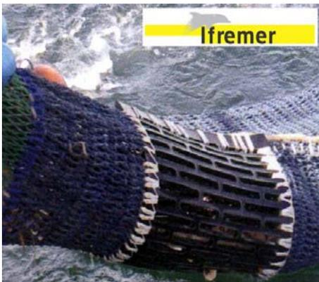
**Figure 8a:** A French design of flexible grid to release *Nephrops* from the belly panel.
