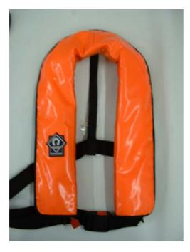
**Product description:** A single chamber halter style lifejacket with a rounded collar. The cover is orange PVC and has zip fastenings. The belt has a plastic 'push lock' buckle and the inflation mechanism is the 'Hammer' hydrostatic.
