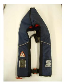
**Product description:** A halter style single chamber lifejacket with a fold down collar that has a fleece comfort strip. The cover is blue fabric secured with Velcro and the belt has a plastic/stainless steel 'push lock' buckle. A clear plastic window covers the inflation mechanism allowing the green indicator to be readily seen. The window is secured with a zip giving easy access to the inflation mechanism.
