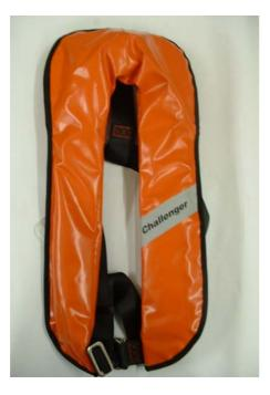
**Product description:** A halter style single chamber lifejacket with a rounded collar. The cover is orange PVC and is secured with Velcro. The belt has a stainless steel 'loop in loop' buckle and is fitted with the optional 'D' ring for attachment of a safety line. This lifejacket has interlocking lobes to combat water flushing into the wearer's face that can occur along the 'V' formed by the lobes on other lifejackets.
