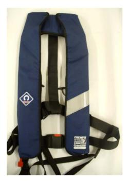
**Product description:** A halter style single chamber lifejacket with a fold down collar. The cover is blue nylon fabric fastened with a zip and has toggles fitted. A crutch strap is supplied but needs to be fitted. The inflation mechanism is 'Hammer' hydrostatic.
