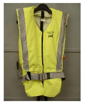
**Product description:** A waistcoat design single chamber lifejacket. The material is day-glow yellow nylon fabric and the waistcoat is fastened with a plastic zip. The belt has a stainless steel 'loop in loop' buckle and a crutch strap is fitted. The waistcoat has two small external pockets and a large internal pocket all fitted with a Velcro sealed flap. Reflective strips are fitted at both sides and front and back. Also, the belt is reflective.
