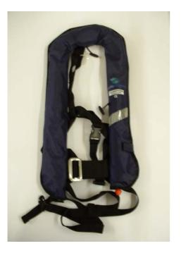
**Product description:** A halter style single chamber lifejacket with a rounded collar. The cover is blue nylon fabric and secured by a zip. Toggles are fitted. The belt has a stainless steel 'loop in loop' buckle and a crutch strap is supplied and fitted.
