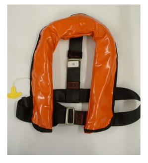
**Product description:** A short length halter style single chamber lifejacket with a rounded collar that is worn high on the chest. The covers are orange PVC and are secured with Velcro. The belt has a stainless steel 'loop in loop' buckle and two options are tried, front and side fastening. This is a new product and a prototype model is shown. (See product No 26, Gael Force Hi-Line Pro for the developed product manufactured by International Safety Limited)
