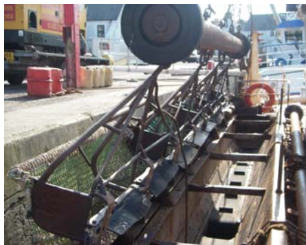
Rubber flappers in various stages of wear and stiffness.
