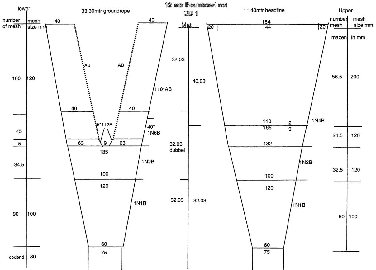
Fig. 1. Net plan conventional beam trawl used on trip 1–3, 8–10.
