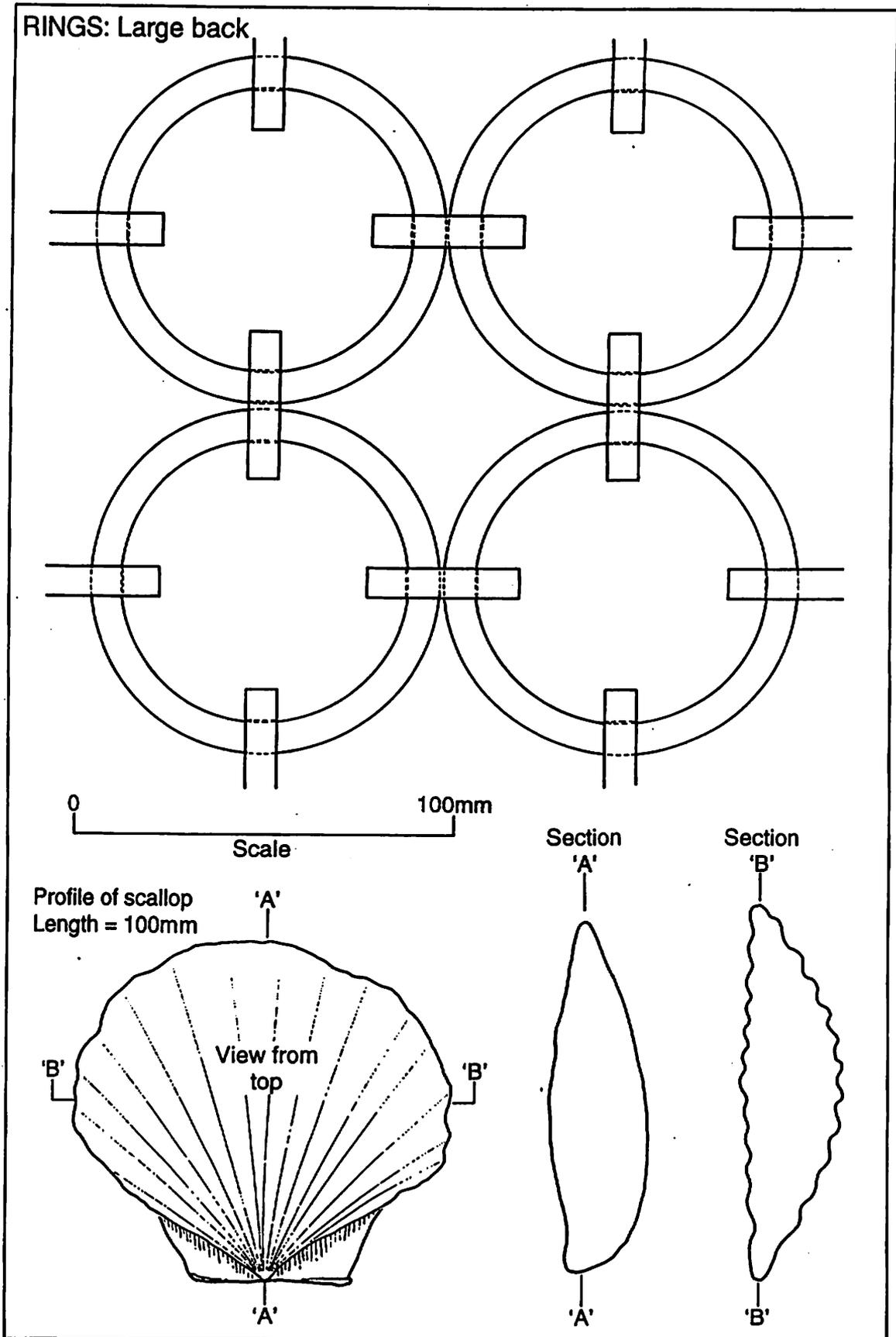
Figure 35: Tooth profile compared with Scallop profile – small tooth spacing
