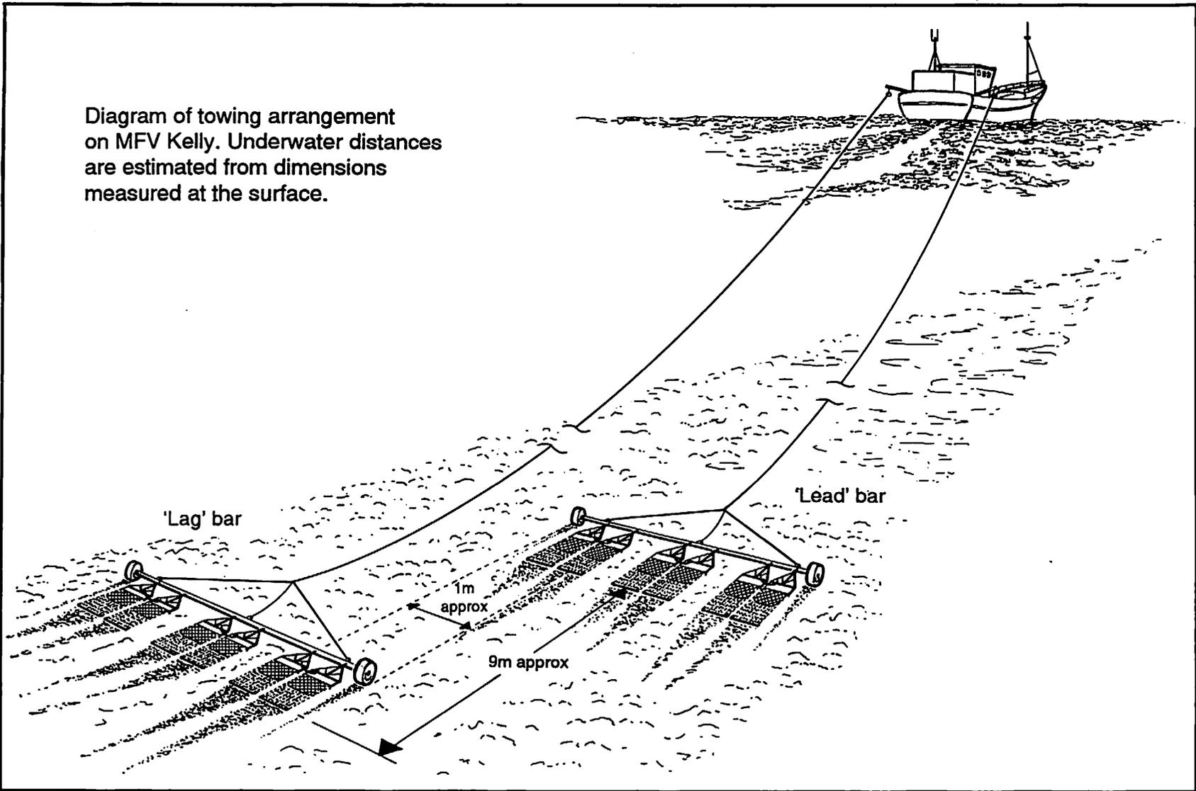
The tooth spacing on all experimental dredges was small on the first day and changed to large on the second but otherwise remained the same. At the end of the second day the experimental dredges were rearranged (Figures 8 and 9, pp20 and 21) so that those which had been inboard on the port dredge were placed outboard on the starboard dredge and *vice versa*. The tooth spacing on all experimental dredges was small for day 3 and large for day 4.
