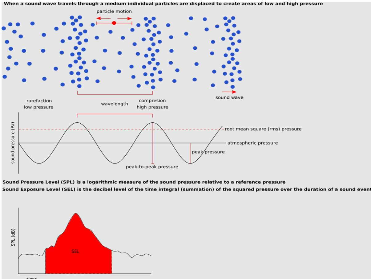
**Figure A8.** Simplified illustration of particle motion and sound pressure measurements.
