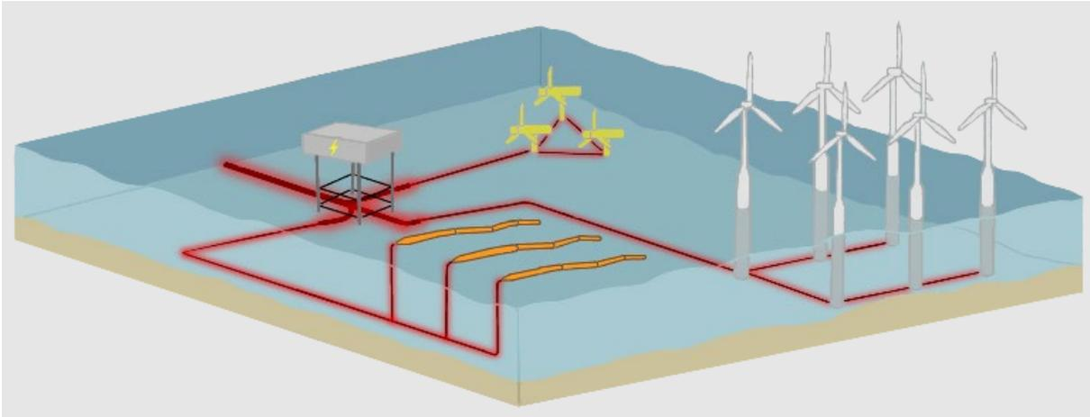
**Figure 2.** Illustration of subsea cables around Marine Renewable Energy Devices (MREDS). © St Abbs Marine Station.
