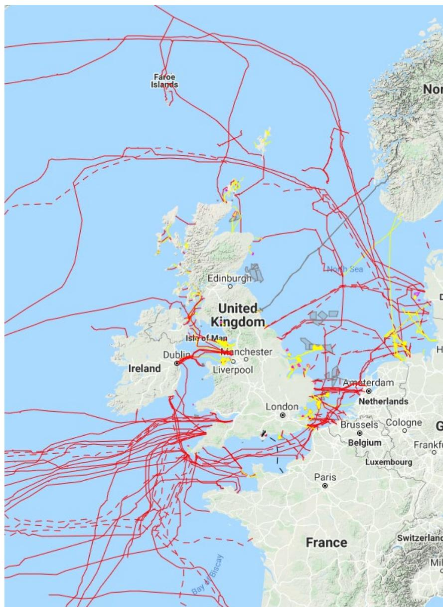
**Figure 3.** Subsea cables found around the United Kingdom. Red = telecommunication cables, yellow = power cables, black = proposed cables. Map produced by Kingfisher Information Service – Offshore Renewable & Cable Awareness project (*From KIS-ORCA*).
