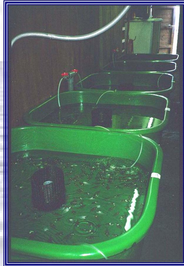
Typical shallow 1m fibreglass halibut weaning tanks
