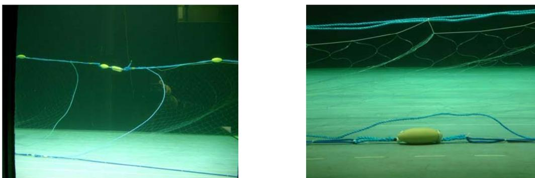
**Figure 1 Pingers in flume tank; left AIRMAR Pinger attached next to a float, right AQUAmark pinger attached to tangle net leadline.**
