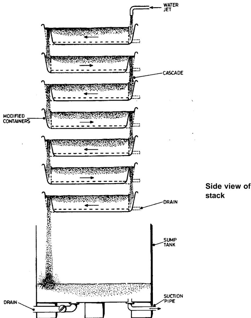
The molluscs are held in purpose designed, solid sided containers which are either directly stacked or supported above one another in a frame over a sump tank. Seawater is drawn from the sump up to one end of the top container of the stack. It passes along the container and then cascades down from the other end into the container below and so on until it returns eventually to the sump.
