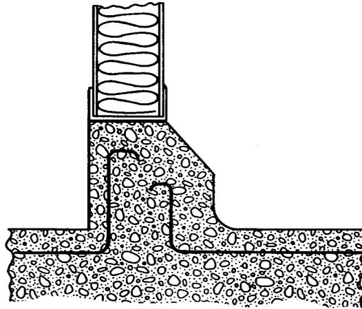
If extended high enough, the upstand protects the wall from impacts by truck forks, pallets, etc., and has the further advantage in storage areas of creating a gap between stacked boxes and the wall to permit the circulation of air.
