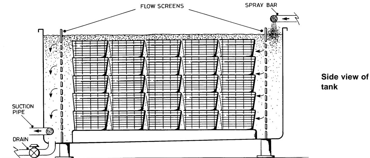
The molluscs are held in mesh type containers stacked up to 6 high in a deep tank. Seawater input is by cascade or jets at one end of the tank. The water passes through a flow-screen to the centre section of the tank containing the molluscs and then passes through a further flow-screen before exiting via a suction pipe.
